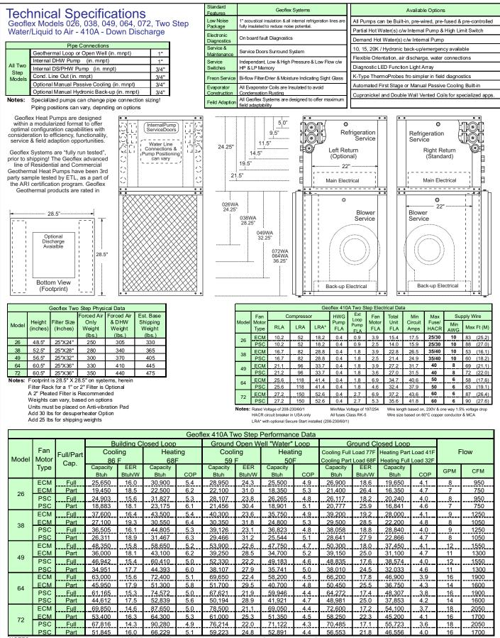
Heating capacities based upon 68°F DB, 59°F WB entering air temperature NOTES: Cooling capacities based upon 80.6°F DB, 66.2°F WB entering air temperature
